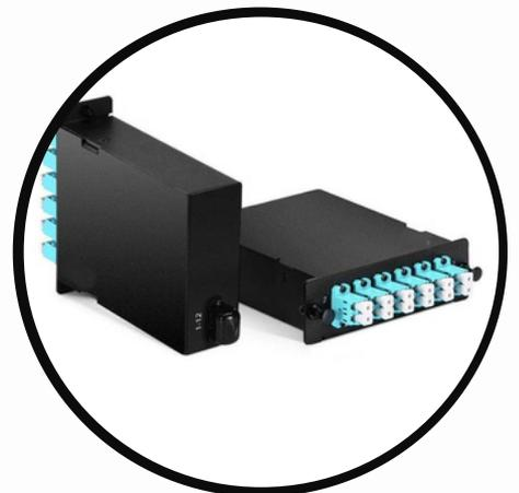
High Density (HD) Cassette (HD ODF), 1 x 12F Mpo (M) to 6 x LC DX, Multimode, Type B
